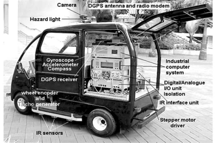
Fig. 11. Mobile robot used in SLAM experiments.
