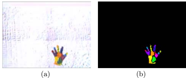
Figure 5: (a) Resultant image after background removal; (b) result of color classification after background removal
