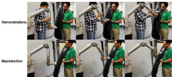
Fig. 5: Painting task on the real Barrett WAM robot. First row shows kinesthetic teaching of the painting task. Second row represents the task reproduction.
