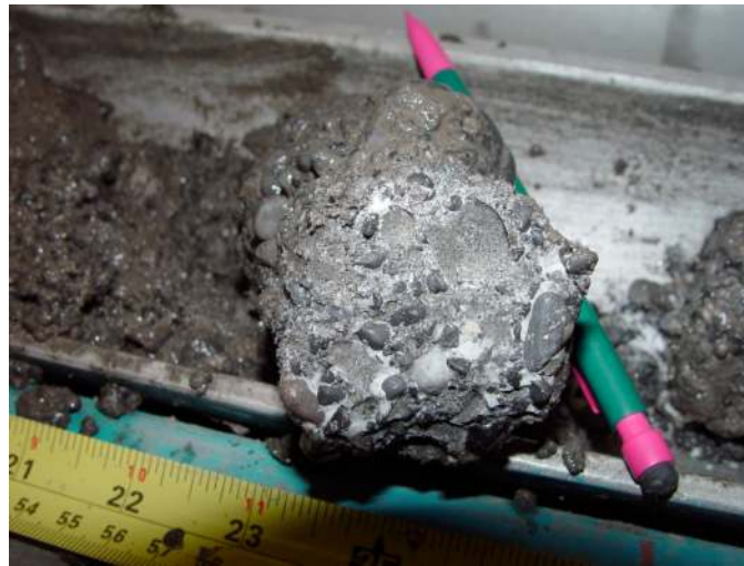
Figure 5 – Photograph of a gas-hydrate-bearing rock core from the Mallik 5L-38 Gas Hydrate Research Well. Note that the gas hydrate is the white material filling the void spaces in this conglomerate (photo courtesy of the Mallik 2002 Gas Hydrate Production Research Well Program - Dallimore and Collett, 2005).
