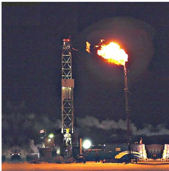
Figure 7 – Photograph of the gas flare from the thermal gas hydrate production test in the Mallik 5L-38 Gas Hydrate Research Well (photo courtesy of the Mallik 2002 Gas Hydrate Production Research Well Program - Dallimore and Collett, 2005).
