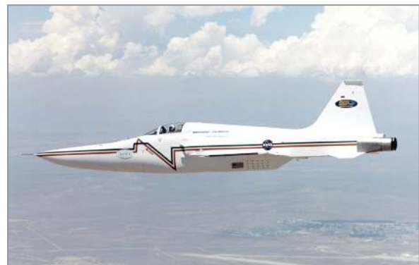
Figure 27 – Photograph of modified F-5E used in SSBD and SSBE flight tests (91).
