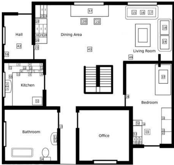
Fig. 2. Plan view of the ground floor of the University of Hertfordshire Robot House. Numbered boxes show the locations of sensors.
