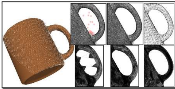
Fig. 10. Processing point clouds. From left to right in the upper part: noisy raw data acquired from the scanner, processed data with the noise removed, resampled point cloud using RMLS. In the lower part their representative polygonal reconstruction.
