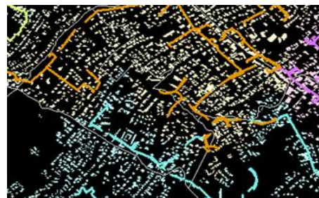
Figure 9: Example of relating building agents and electrical lines (from GIS). Building agents are geo-referenced and connected by proximity to the closest infrastructure line (same colours).
