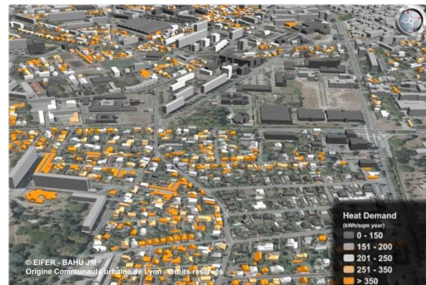
Figure 3: Representation of the heat demand results of residential buildings considering the scenario A “construction state”.
