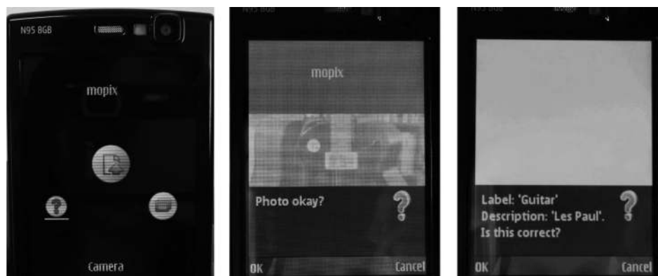
Fig. 1. The mopix phone application interface to access the camera, help page and gallery, which shows all of the photos the user has taken, both shared and unshared (left). After taking a photo, the user is prompted to share the photo (center). If shared, the user is asked to provide a title and description for the photo (right).
