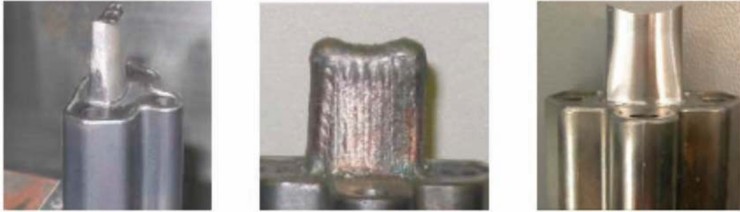
Figure 7: Worn Die that was Repaired (Ren et al. 2006)
