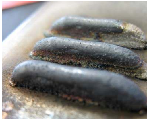
Figure 2.3: Thin Walls Built by Computer Control
