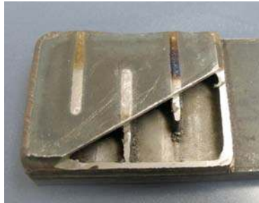
Figure 9: Part with Cooling Channel
