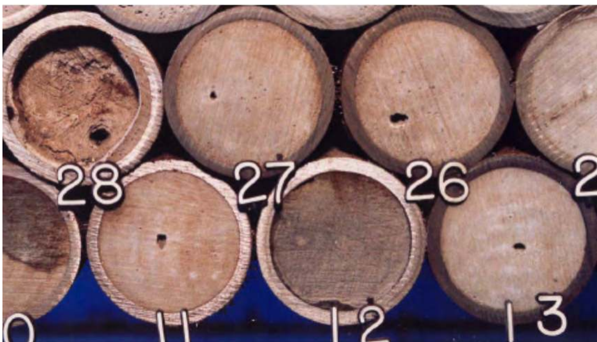
Figure 3.5. Channels and gas pockets formed as a result of gas invasion during cementing set (from Watson, 2004)
