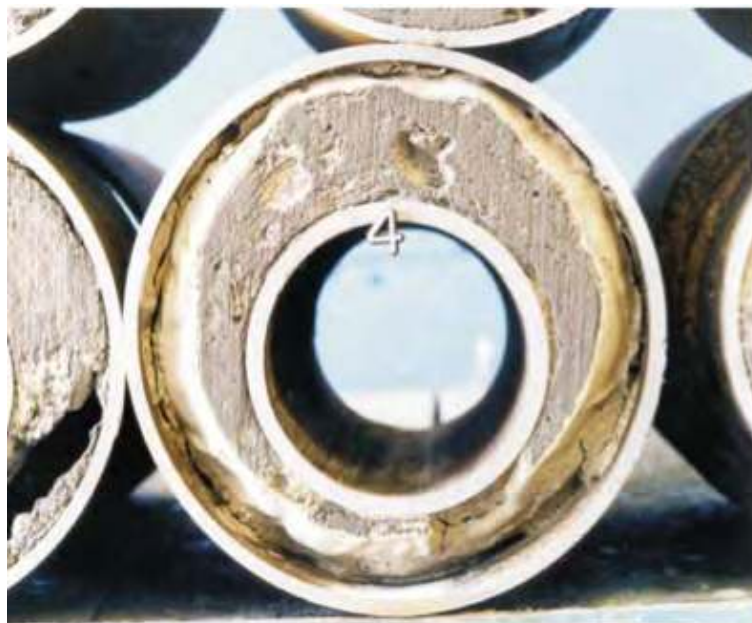
Figure 3.3. Cement and drilling fluid channels resulting from incomplete drilling mud displacement. Note that because of the eccentric casing, the severity of the problem on the thinner annulus is much greater (from Watson, 2004)
