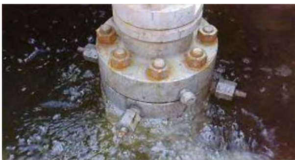
Figure 6.2. Bubbling of standing water surrounding a wellhead, from Ingraffea (2011)
