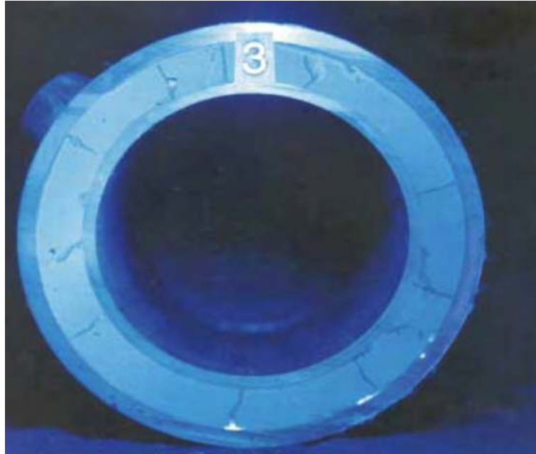
Figure 3.6. Cement sheath failure and crack development as a result of pressure cycling (Watson, 2004)
