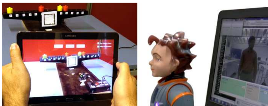
Fig. 4. The Zeno robot, the EASELscope and the Smart Balance Beam (SBB). Zeno acts as the embodiment of the STA and continuously interacts with the learner. Information about the task is displayed as augmented reality on top of the physical SBB.
