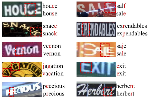
Figure 6. Right cases of SRN with/without GSRM. The predictions are placed along the right side of images. The top string is the prediction of SRN without the GSRM; The bottom string is the prediction of SRN.
