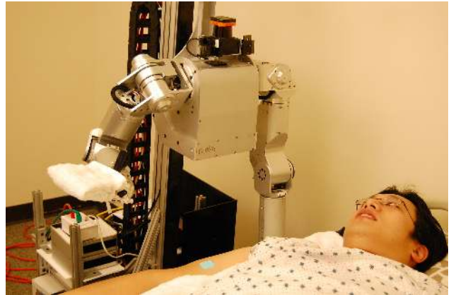
Fig. 1. Experimental Setup: The robot Cody was situated along side the patient bed, ready to perform the cleaning task to a subject (IRB approval and user permission obtained).
