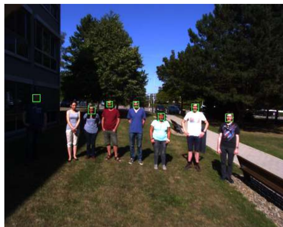
Figure 14. Direct sunlight example: note the detection of the person standing in the shadow.
