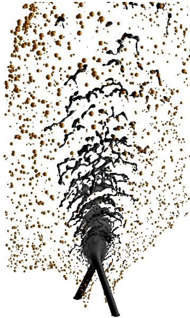
Figure 11. Isometric view of the impinging jets at t = 7.659 ms.
