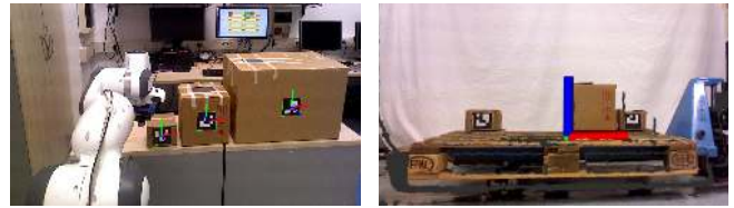
Fig. 3. (left) Box frames detected by the ArUco marker detector using the RGB images from the ASUS camera. (right) Coloured point-cloud acquired by the Orbbec camera. The frame has been placed in the centre of the top surface of the pallet, after detecting the three wooden blocks.
