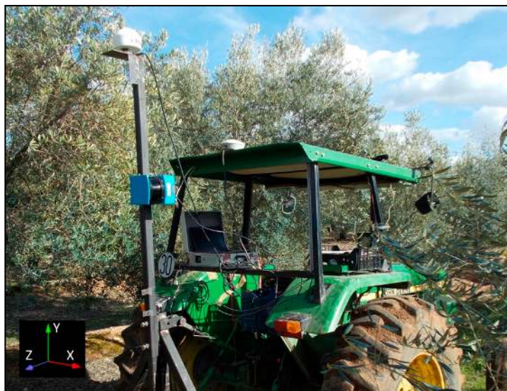
Figure 5. LiDAR sensor and laptop computer in the field, installed on the tractor.
