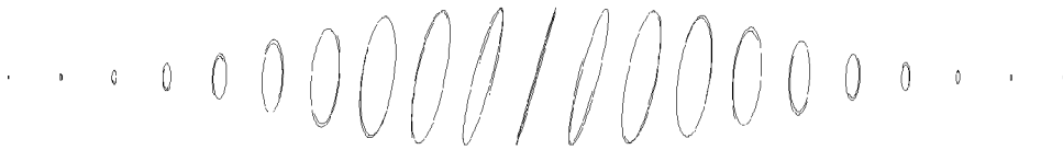
Fig. 12. Polarization chirp produced by superposing two Gaussian pulses linearly polarized along two orthogonal directions and with a temporal delay equal to half their duration. The polarization is linear only for a fraction of the pulse around its maximum.
