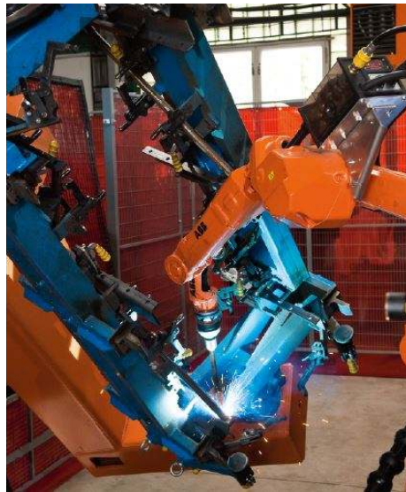
Figure 12: Welding of hoist machinery carried out by robot – Adapted from O'Connor (2008)
