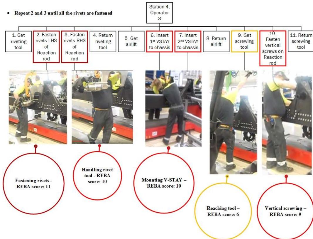
Figure 28: HTA showing the main goal, sub-tasks and REBA scores for Operator 3 at workstation 4
