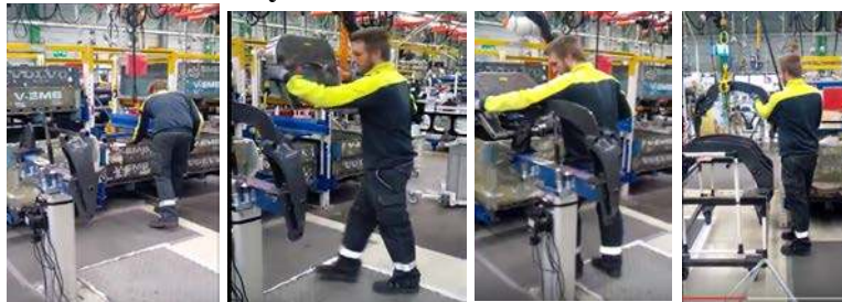
Figure 7: a) Get component b) Getting rivet tool c) Horizontal riveting d) placing subassembly
