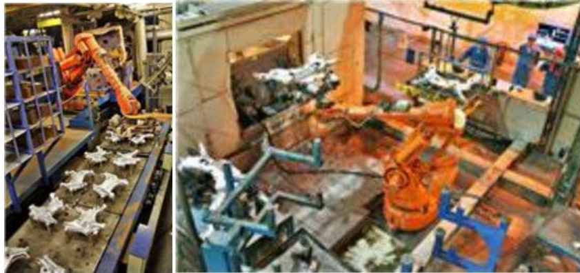
Figure 11: Robots picking and placing automotive components during sand casting – Adapted from Fouché (2010)
