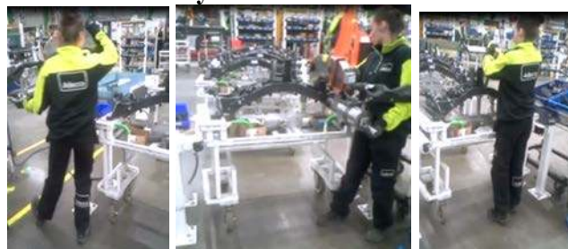
Figure 5: a) Grabbing riveting tool b) Horizontal riveting c) Screwing
