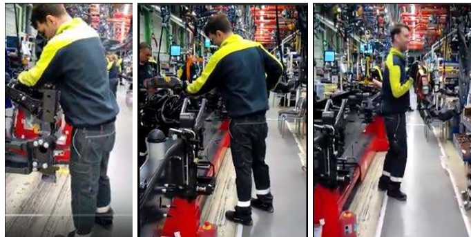
Figure 3: a) Riveting vertical b) Riveting horizontal c) Grabbing riveting tool
