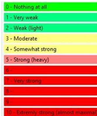
Figure 16: Borg scale of perceived exertion - Adapted from "AviX Ergo - Is used to improve the ergonomics of the workplace" (2016)
