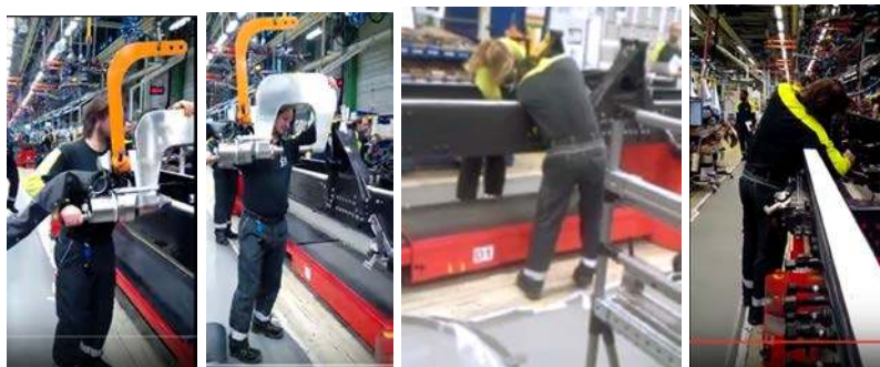
Figure 4: a) Horizontal riveting b) Grabbing tool c) Inserting V-STAY d) Screwing
