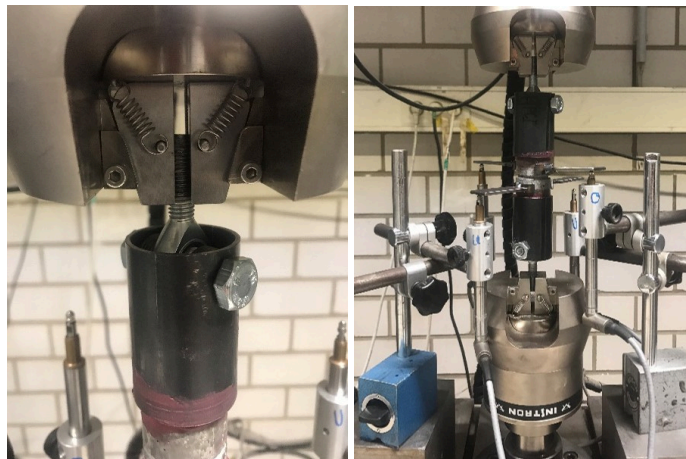
Figure 1: Load application (left) and tensile test bench (right)
