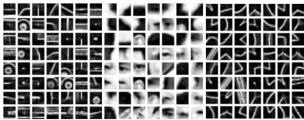
Figure 3. A sample of the patterns obtained from our feature selection method (based on k-means clustering) is shown for cars (left), heads (center) and leaves (right). The leaf and car images were high-pass filtered before feature selection. The total number of patterns selected was 175 for heads (across a 90^\circ range of viewing directions), 89 for cars (across two orthogonal viewing directions) and 81 for leaves.
