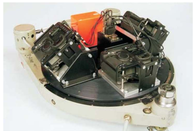
Fig. 1 DLR 3K-camera system consisting of three Canon EOS 1Ds Mark II, integrated in a ZEISS aerial camera mount, and an IMU (red box)
