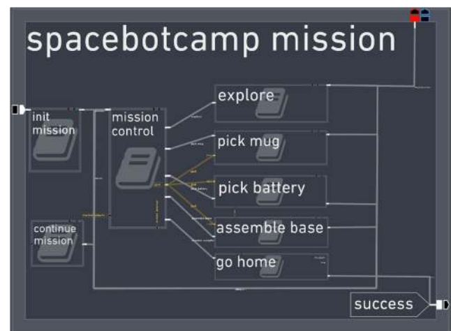
Fig. 24 Simplified SpaceBotCamp top-level state machine containing a single decision state, mission control , that decides on which sub-plan to execute next based on the current world state and a set of rules. This structure allows for a flexible course of action and simplifies error handling and human interaction. The pick mug state depicted in this screenshot refers to the state for picking up the rock sample
