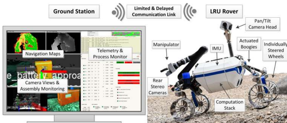
Fig. 2 System overview showing the key components of the ground station GUI for monitoring and the rover hardware modules
