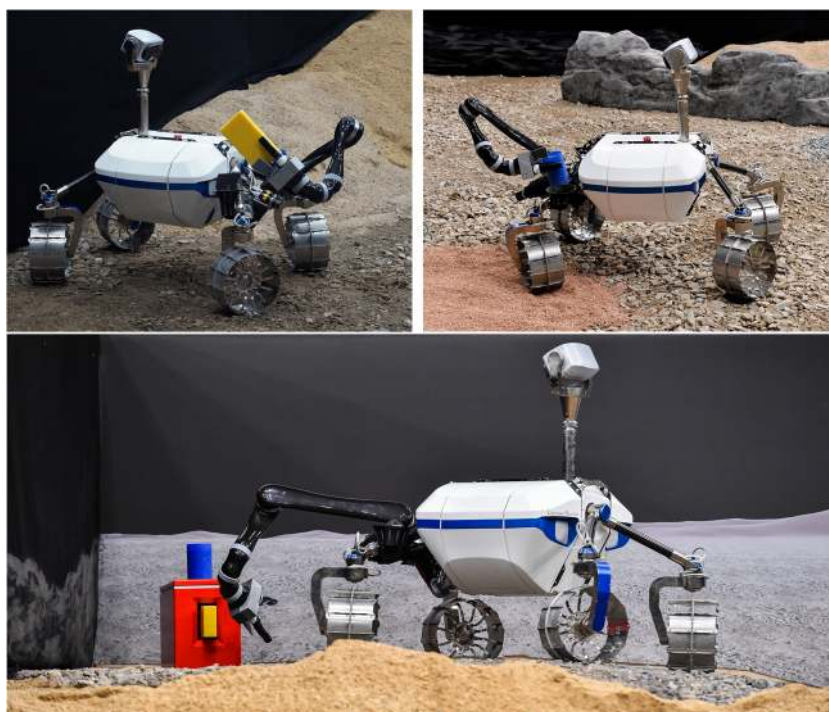
Fig. 1 Our Lightweight Rover Unit (LRU) picks up the battery (yellow, top left) and the sample (blue container, top right) and assembles them at the base station (red, bottom) during the SpaceBotCamp challenge
