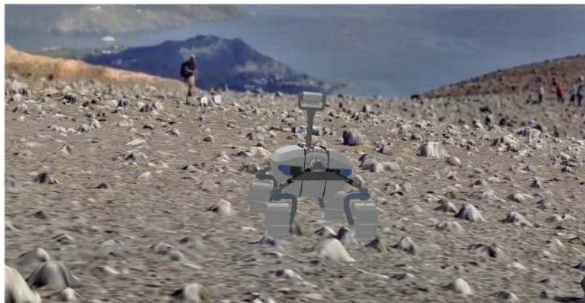
Fig. 29 Simulation of the LRU at a hillside on Vulcano, Italy. Ground reconstructed based on laser scans and panoramic images
