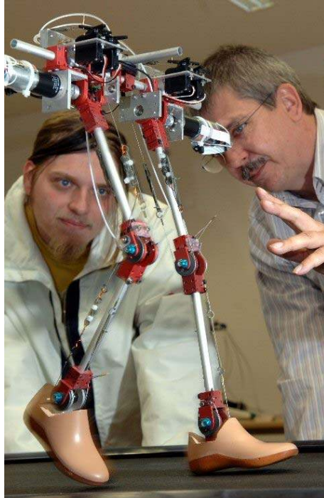
Figure 1: The JenaWalker II bipedal robot testbed.
