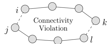
Fig. 4. Control challenges due to multiple link deletions. In the absence of an agreement protocol, simultaneous deletion of links (i, j) and (k, l) violates connectivity.
