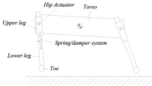
Figure 3. Scout II mechanical system
