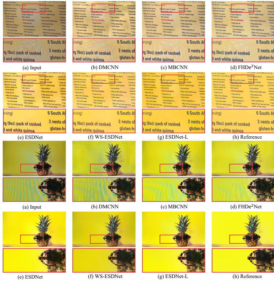
Fig. 13: Qualitative comparisons of our models with three representative state-of-the-art methods on the FHDMi dataset [13], including DMCNN [13], MBCNN [47] and FHDe 2 Net [13]. ESDNet is our standard model and ESDNet-L is our larger model. WS-ESDNet is our more lightweight model, the parameters of which are shared in three branches of pyramid context extraction module
