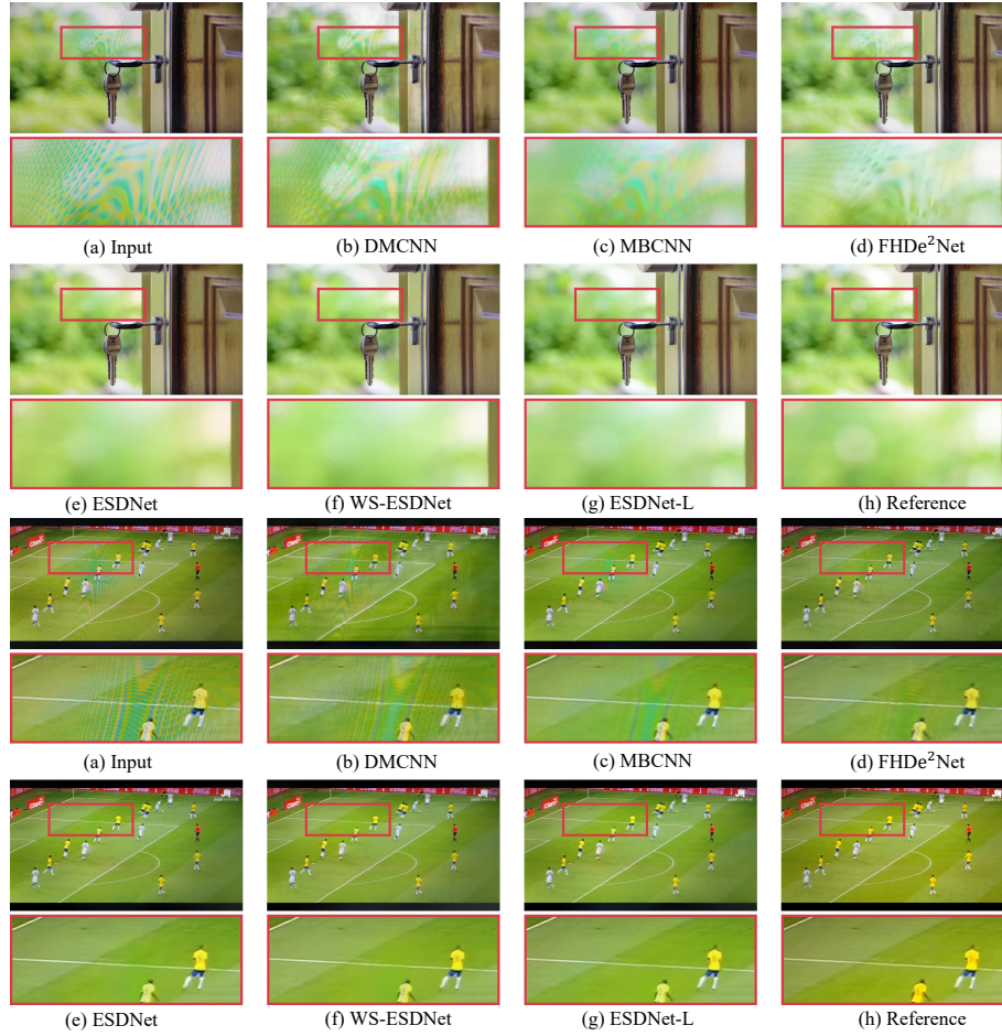
Fig. 12: Qualitative comparisons of our models with three representative state-of-the-art methods on the FHDMi dataset [13], including DMCNN [29], MBCNN [47] and FHDe 2 Net [13]. ESDNet is our standard model and ESDNet-L is our larger model. WS-ESDNet is our more lightweight model, the parameters of which are shared in three branches of pyramid context extraction module
