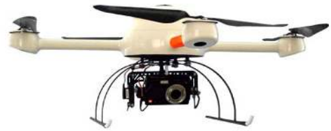
Figure 1: Micro-drone md4-200 with attached PENTAX Optio A40.
