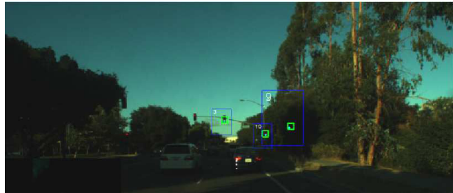
Fig. 7. Simultaneous detection of three distinct traffic lights at one intersection. The left turn lights do not affect our lane, so are not considered.
