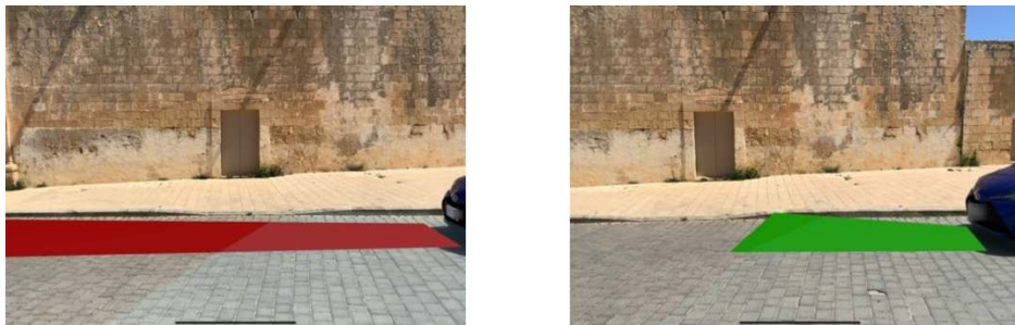
Figure 4: Concept 4. Left : non-yielding state with the red field of safe travel extending over the crossing area. Right : yielding state with the green field of travel shortened and truncating before the crossing area.
