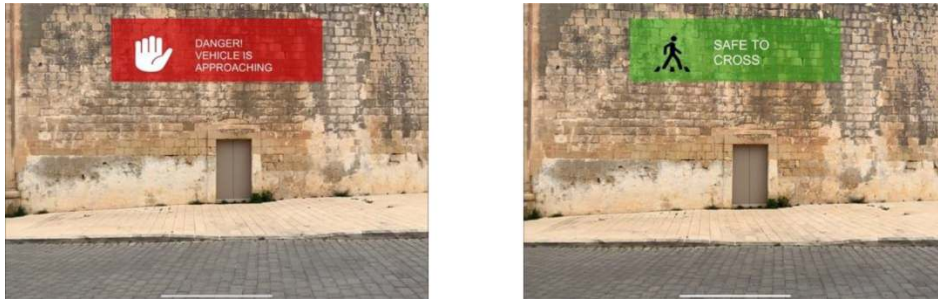
Figure 8: Concept 8. Left: the non-yielding state with the red HUD showing the hand icon and corresponding text message. Right: the yielding state with the green HUD, walking pedestrian icon, and corresponding text message.
