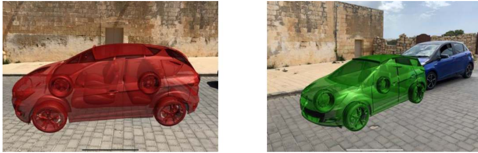
Figure 7: Concept 7. Left: non-yielding state with the red phantom car blocking the crossing area. Right: yielding state with the real car entering the green phantom car.
