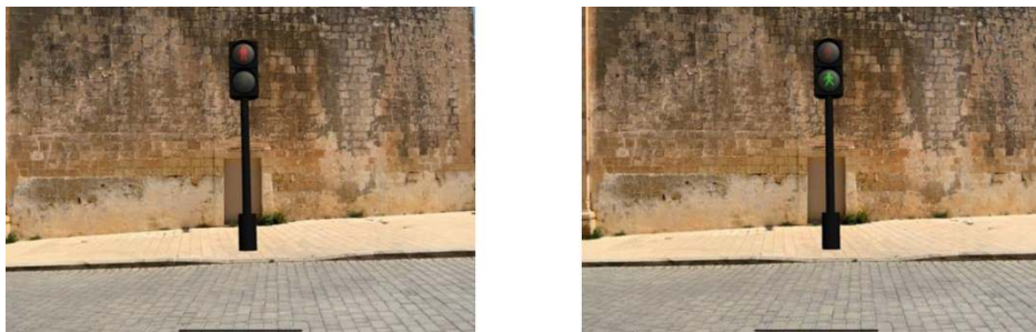
Figure 5: Concept 5. Left : non-yielding state with red pedestrian icon. Right : yielding state with green pedestrian icon.
