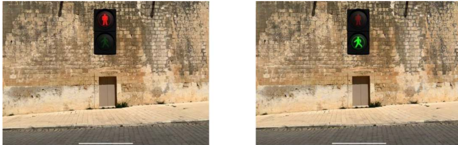
Figure 9: Concept 9. Left: non-yielding state with the red pedestrian icon. Right: yielding state with the green pedestrian icon.
