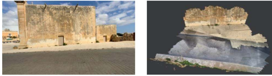
Figure 1: Left: The chosen unmarked crossing in Malta. Right: The captured LiDAR 3D scan on location.
