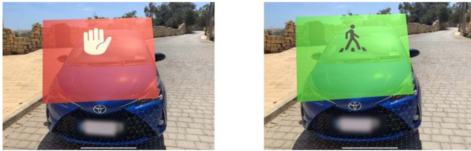
Figure 3: Concept 2. Left : non-yielding state with the red plane and hand icon augmented on the vehicle. Right : yielding state with the green plane and crossing figure icon augmented on the vehicle.
