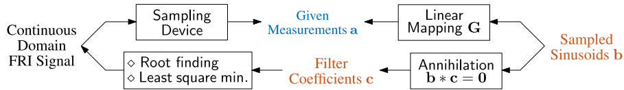
Fig. 4. Overview of the generic FRI reconstruction problem. The continuous domain FRI signal is reconstructed from the given measurements \mathbf{a} by enforcing the annihilation constraint on the unknown sampled sinusoids \mathbf{b} , which are related with \mathbf{a} via a linear mapping \mathbf{G} .
