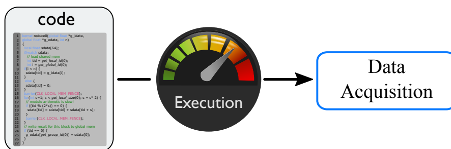
Figure 4.2: Data for the visual exploration of parallel programs is acquired either from the plain source code, or using recordings during the execution of the program.
