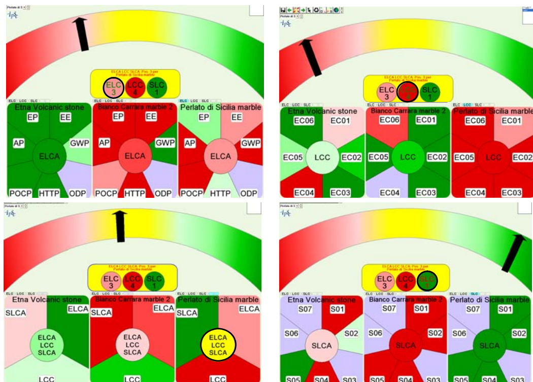
Figure 5. LCSA graphical scheme; individual results for LCA, LCC and SLCA in the upper part and lower right; overall LCSA result in the lower left; example shown is a comparison of different hard floor coverings.
