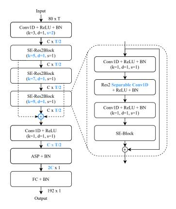
Fig. 2. Network topology of ECAPA-TDNNLite. k denotes kernel size, d denotes dilation rate and s denotes stride in Conv1D layers and SE-Res2Blocks. C and T are the channel and time dimensions of feature mappings, respectively. Modifications in comparison with ECAPA-TDNN are plotted in bold blue.
