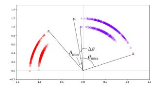
**Fig. 3.** Explanation for effectiveness of the asymmetric structure.  $\times$  and  $\triangle$  denote speaker embeddings extracted by ECAPA-TDNN and ECAPA-TDNNLite, respectively. The two speakers are plotted in different colors.
