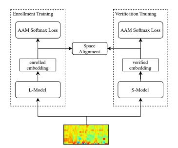
**Fig. 1.** The training process of the asymmetric structure. Frame-wise input features are fed into the large-scale model and the small-scale model, respectively. AAM softmax loss is applied on both enrollment and verification sides, and an additional loss function aligns the speaker subspace bewteen the enrolled embeddings and the verified embeddings.
