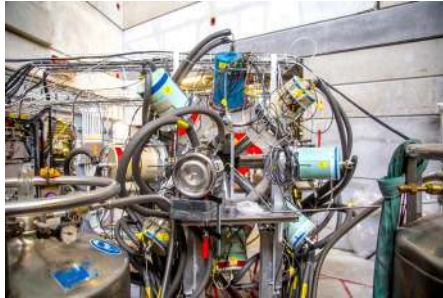
Fig. 1. – Setup for the test of muon transfer reactions in a high-density-deuterium gas mixture at the \pi E1 area at PSI. The gas target is placed at the center of the detector array.
