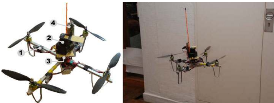
Fig. 24 Our quadrotor ( left ): 1 Mikrokopter platform, 2 Hokuyo laser range finder, 3 XSens IMU, 4 Gumstix computer. Right Our system during a mission
