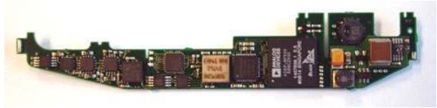
Fig. 18 The IMU of muFly. The elongated shape imposed strong constraints on the analog chain design
