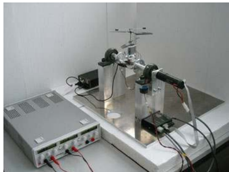
Fig. 2 Schematic layout of the stabilizer test-bench (left), and photo of the test-bench at the ASL (right). A lab power supply is used for powering the motors and the electronics
