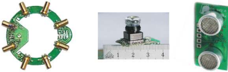
Fig. 9 Position sensors. Combined laser diodes ( left ) and omnidirectional camera ( center ), ultrasonic range finder ( right )
