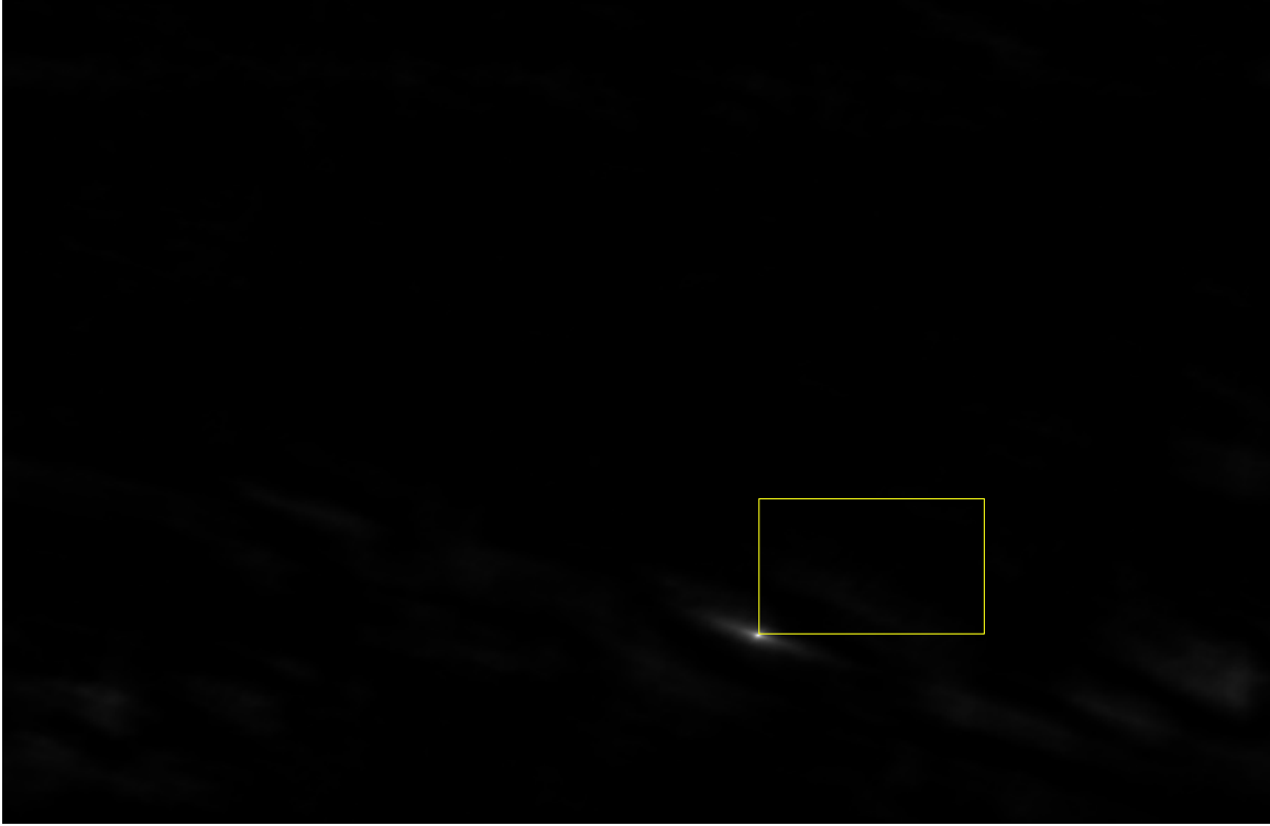
Figure 3. The correlation function computed for the truck template and the image shown in Figure 2. Lighter grayscale indicates larger values. There is a unique maximum, at the offset corresponding to the location of the template in the image.
