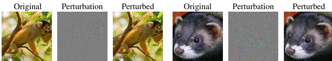
Figure 7: AIP for an ImageNet classifier. The perturbations are generated at L_2 = 1 \times 10^{-4} .
