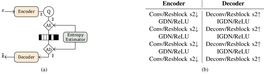
Fig. 3: Neural Image Compression (NIC) . (a) Basic architecture of VAE-based NIC Solutions. Q denotes the quantization. The entropy estimator provides the probability estimation for both AE (Arithmetic Encoding) and AD (Arithmetic Decoding); x is the input source image, and correspondingly \hat{x} is the output reconstruction (after decoding). (b) Typical paired Encoder and Decoder components used in NIC framework, such as normal Convolutional layer (Conv) or ResNet block (Resblock) [30], resolution re-sampling (upsampling s2\uparrow and downscaling s2\downarrow at a factor of 2), nonlinear activations using GDN (Generalized Divisive Normalization) [31] or ReLU (rectified linear unit) [32]. Deconv and IGDN are inverted processes of respective Conv and GDN.
