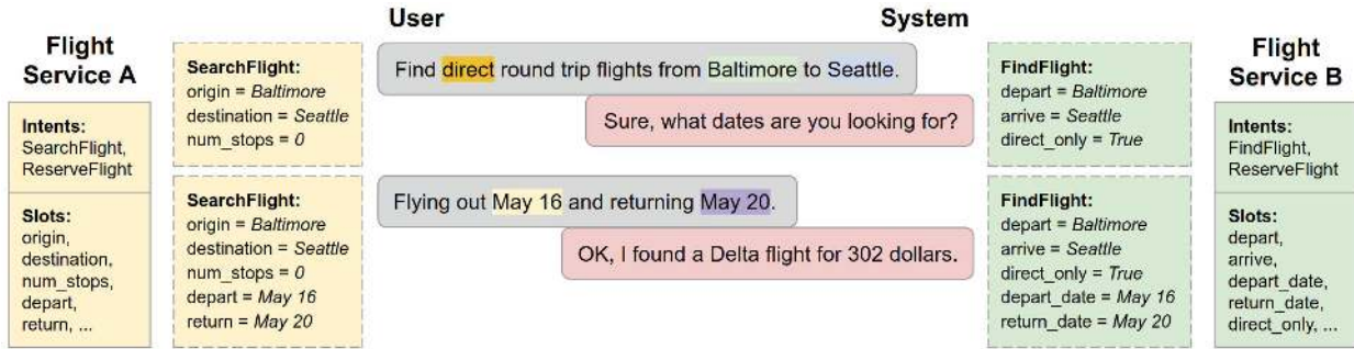
Figure 5: The predicted dialogue state (shown with dashed edges) for the first two user turns for an example dialogue, showing the active intent and slot assignments, with two related annotation schemas. Note that the dialogue state representation is conditioned on the schema under consideration, which is provided as input, as are the user and system utterances.
