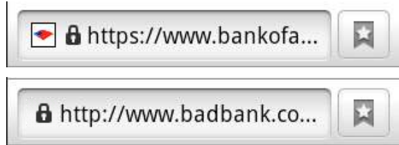
Figure 8: The address bar of the Android browser when a webpage over SSL is loaded. The browser places the favicon adjacent to the lock icon, thereby violating the W3C guideline 3b described in Section 4.2.2. The star icon to the right of the address bar is to bookmark the webpage.
