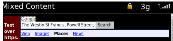
Figure 6: Blackberry Mango browser rendering a mixed content webpage. Note that the webpage contains a Google map obtained over an http connection. Although the webpage holds mixed content, the browser displays the padlock icon as well as the https URL prefix indicators. This behavior fails to meet with guideline 3a.
