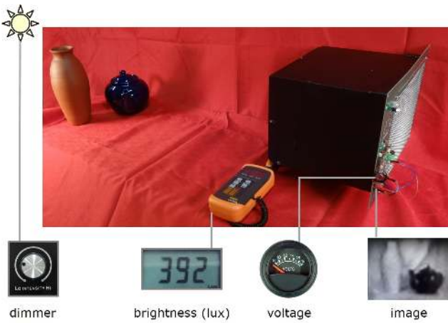
Figure 12. The setup used to evaluate the power performance of the camera.
