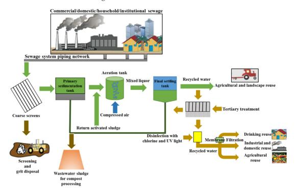
Figure 2. Water-reclamation process at the treatment facility modified from [60,61].
