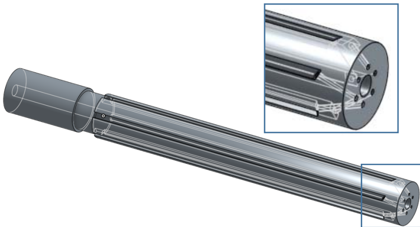
Figure 3. Ceramic insulator with propellant feed channels.
