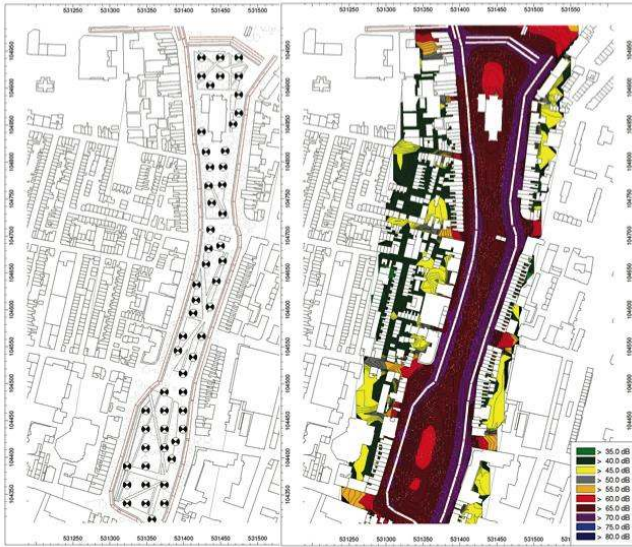
Figure 14: Valley Gardens. Identification of receiver points (left). L_{den} values with updated traffic data (right).
