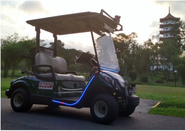
Fig. 1. The autonomous golf cart equipped with LED strip [36]. The blue color indicates no obstacle within close range, whereas red shows presence of a nearby obstacle.
