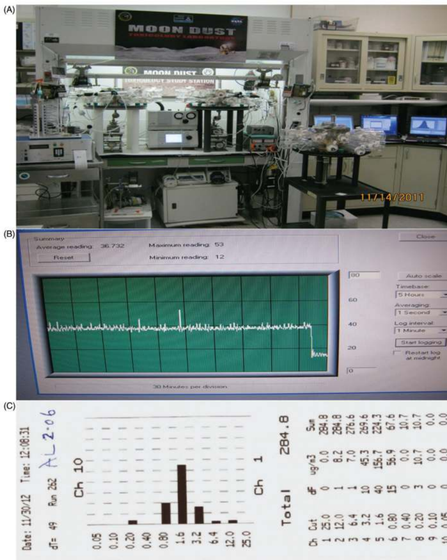
Figure 1. (A) Nose-only inhalation chamber systems and the associated dust generators, cyclones, dust monitors and data acquisition computers. (B) A typical 6-h chamber concentration recorded by the Casella Microdust Pro. (C) An example of a particle size profile recorded by the Quartz Crystal Microbalance Cascade Impactor.
