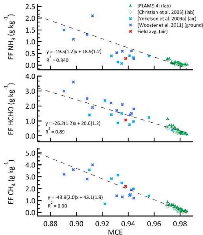
**Figure 4.** Emission factors ( $\text{g kg}^{-1}$ ) of select smoldering species as a function of MCE for FLAME-4 burns of African savanna fuels. Also shown are laboratory data of Christian et al. (2003), ground-based data of Wooster et al. (2011), and airborne data of Yokelson et al. (2003a). The linear fit based on all data is shown.
