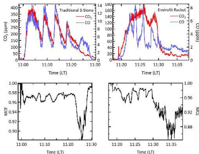
**Figure 9.** Excess mixing ratio profiles of CO and  $\text{CO}_2$  for both a traditional three-stone cooking fire (104) and a more advanced “rocket” design stove (115) showing cleaner combustion and shorter time to reach a steady state in the stove. The profiles of MCE vs. time are included for both stove types.
