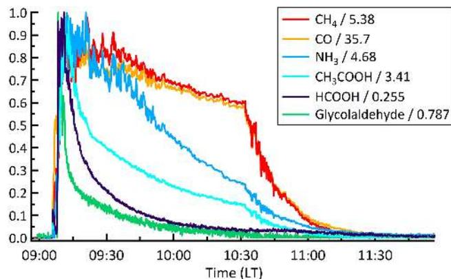
**Figure 3.** Excess mixing ratios of sticky and non-sticky gases normalized by their maximum mixing ratio (shown in legend) to have a maximum value of one during a “room” burn of organic hay. The stable non-sticky species shown are CO and CH<sub>4</sub>, while the stickier species include HCl, NH<sub>3</sub>, glycolaldehyde, CH<sub>3</sub>COOH, and HCOOH; the latter show a faster rate of decay than the stable species CO and CH<sub>4</sub>.
