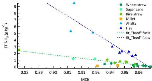
**Figure 11.** Emission factors of  $\text{NH}_3$  as a function of MCE for “feed” crop residue fuels (triangles), “food” crop residue fuels (circles), and older millet samples (squares). Also shown are the lines of best fit from food fuels (green) and feed fuels (blue).
