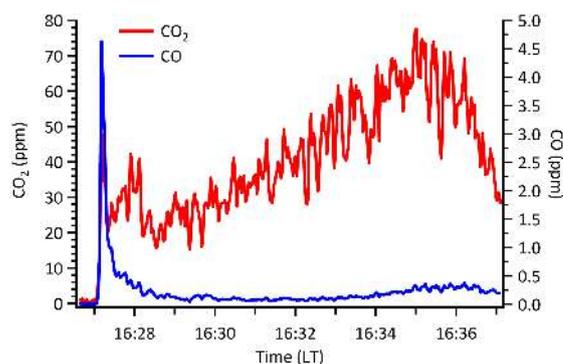
**Figure 13.** Excess mixing ratio profiles of CO and  $\text{CO}_2$  for the FLAME-4 plastic bag burn characterized by a large long-lived ratio of  $\Delta\text{CO}_2 / \Delta\text{CO}$  corresponding to strong flaming combustion.
