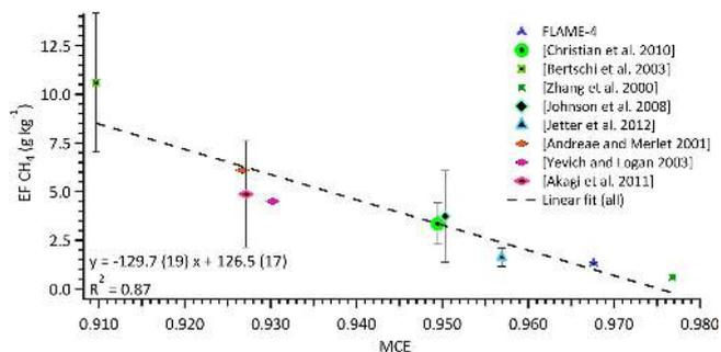
**Figure 10.** Open cooking fire, fire-averaged emission factors of  $\text{CH}_4$  as a function of MCE for current and past laboratory and field measurements together with the recommended global averages. Error bars indicate one standard deviation of the EF for each study where available.
