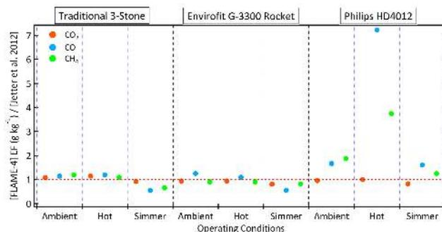
**Figure 8.** Comparison of FLAME-4 three-stone, Envirofit G-3300 Rocket, and Philips HD4012 cookstove EFs to EFs reported during performance testing by Jetter et al. (2012). The EzyStove was not tested by Jetter et al. (2012). Each circle represents the FLAME-4 fire-averaged EF of all fuel types measured with all components starting at ambient temperatures compared to the Jetter et al. (2012) data collected under regulated operating conditions.
