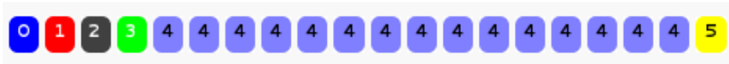
FIG. 10 – Use case 1 : initialization sequence at slices 0-3 followed by a steady state part (4)
